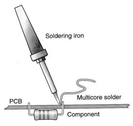
Always place the component as close to the PCB as possible, unless the text in this manual advises otherwise. Next place the PCB upside down on a solid surface. Place the multicore solder between the soldering iron and the leg of the component and gently push the soldering iron against it.
