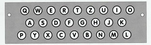
The film can be held in place, by creating a sandwich construction. Find two pieces of transparent plastic or plexiglass, and cut them to the same size as the lamp panel film. Fit the film in between the two pices of plastic and use spacers to fit the lot to the mounting holes in the PCB.
