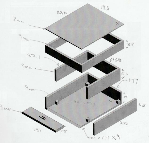
This one is easy to reproduce and looks very much like the original Enigma case. It consists of two parts: a bottom part, containing the main PCB and the Steckerbrett, and the lid. On the next pages you'll find the dimensions, in case you want to give it a go.
