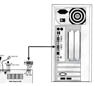
At the PC end, any standard terminal emulation program can be used, such as HyperTerminal for Windows. Any text typed on your **Enigma-E**, will appear enciphered on the PC and vice versa.
