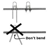
Next we solder the 5 red LEDs (LED1, LED2, LED3, LED4 and LED5), left of the displays. The longest leg should go into the rightmost hole (square pad).
